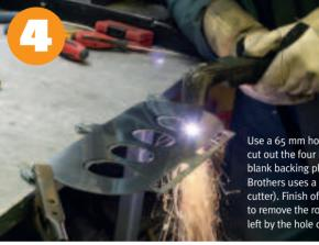
Use a 65 mm hole cutter to cut out the four holes in the blank backing plate (Bogg Brothers uses a plasma cutter). Finish off with a file to remove the rough edges left by the hole cutter.
