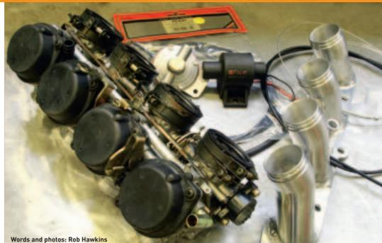
range of motorbike carburettors have been fitted to various car engines, including those from the Honda Fireblade, Blackbird, Kawasaki ZX range and Suzuki Bandit. In this workshop, we're concentrating on the four carbs fitted to the Yamaha R1. These have 40 mm chokes with 1.3 mm diameter main jets. They can't be used to properly fuel a car engine until the main jets have been opened up (see the step-by-step stripping guide for full details).
