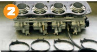
To fit the air filter backing plate, you need the standard R1 backing plate from the air box - or you can make one using a piece of cardboard. You'll also need a set of air box rubbers and clips from a bike breakers or Yamaha dealer.
