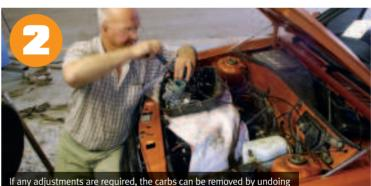
four jubilee clips to access the mixture screws and main jets. The mixture screws need to all be set the same. The main jets can be changed for larger or smaller boreholes.
