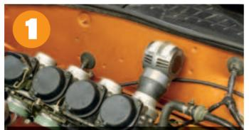
Dave Bogg starts setting up the carbs by checking the fuelling pressure to ensure there's a sufficient fuel supply. Then he checks and resets the balance using an airflow meter, followed by the CO at 3000 and 5500 rpm.
